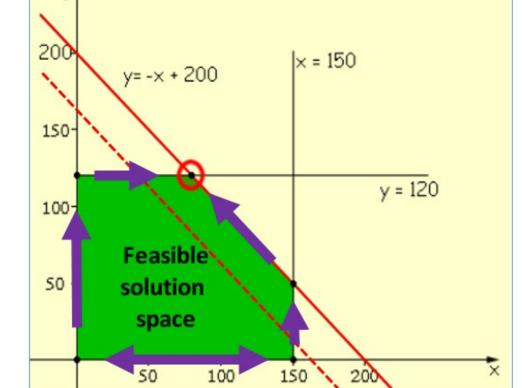
The dotted red line would apply to a scenario where the two generators could not supply the 200 MW needed for load. The model would find an optimal solution in the same manner, minimizing the amount of penalty it must pay. If the requirement to meet load was modeled as absolute, the solution would be infeasible.
