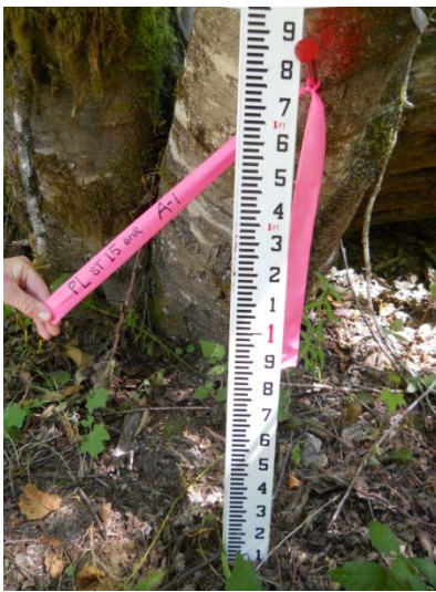
Figure 7 An example of cross-section benchmarks, flagging and rod placement
