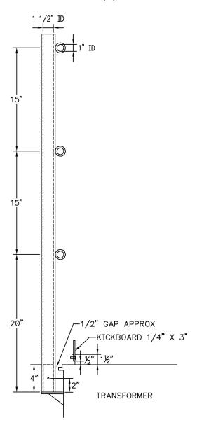
Figure 4—Safety Railing Post and Kickboard Detail
