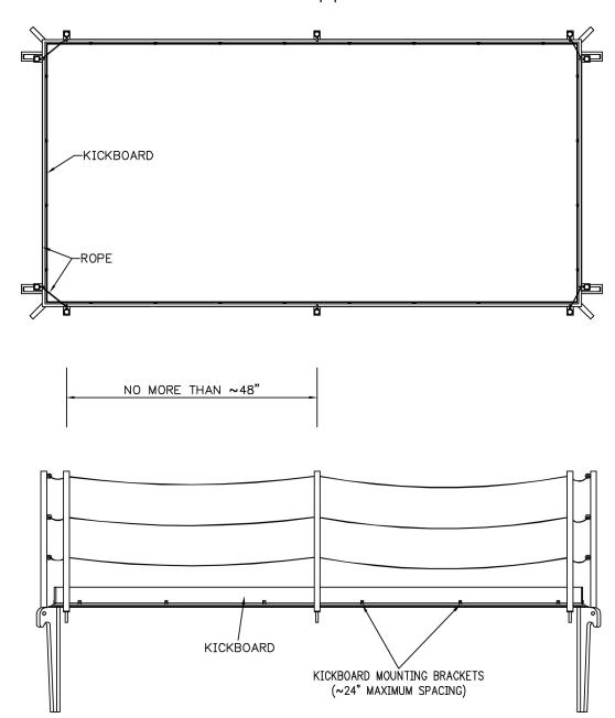
Figure 3—Safety Railing System Overview
