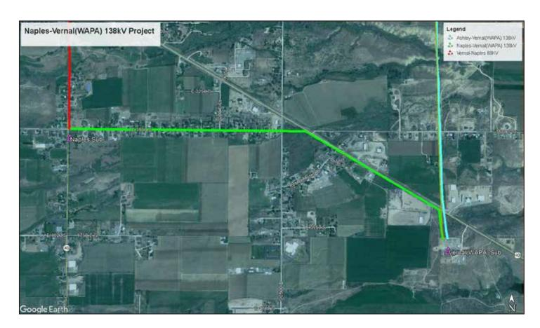
transmission line will follow an existing distribution line on the south side of 3500 South east to State Hwy 40 then follow Hwy 40 to the WAPA substation near Hwy 40 and 3100 E connecting to the Western Area Power Administration Substation. This new line and substation will increase local electric capability and provide for alternate paths for continued service during maintenance and severe weather.
