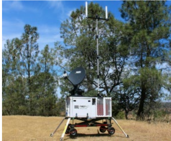
Figure 47: Rapidly Deployable Cell on Wheels
