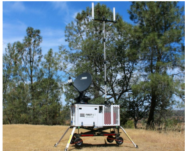
Figure 33: Rapidly Deployable Cell-on-Wheels (COW)
