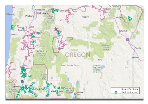
Figure 23: Fault Indicators Installed in 2022
