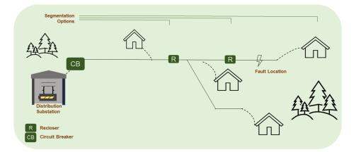
Figure 33: Example of Distribution Circuit with Multiple Reclosers 80 of 160
