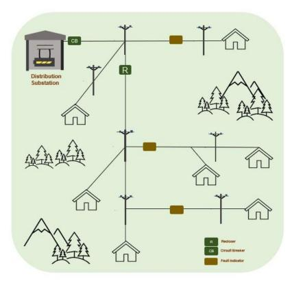
The time it takes to patrol a line and overall impact to customers can be substantially reduced when the fault location can be determined. Therefore. as described in Section 4.4 and generally depicted in Figure 35, Pacific Power installed fault indicators in 2022 across the Oregon service territory, prioritizing circuits that fed into the FHCA areas where EFR settings are most likely to be implemented. When an outage occurs, these new tools are
