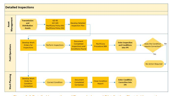
Figure 8-2 Detailed Inspections of Transmission and Distribution Electric Lines and Equipment Workflow
