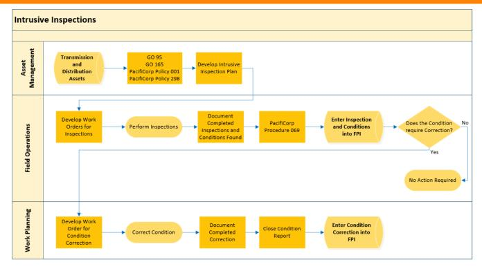
Figure 8-3 Intrusive Pole Inspections Workflow
