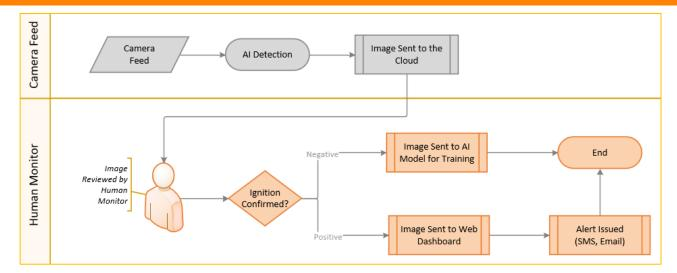
Figure 8-16 Camera Data Flow Diagram
