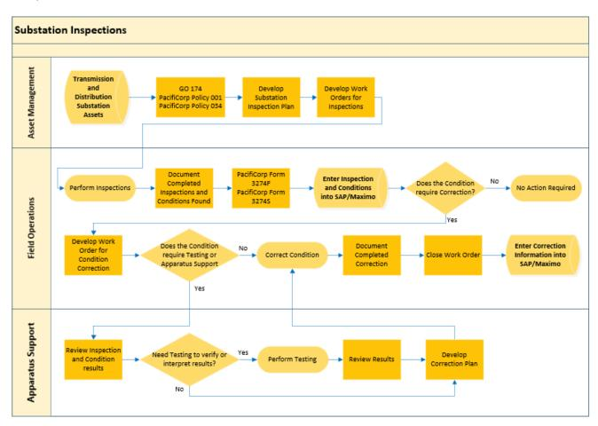
Figure 8-4 Substation Inspections Workflow
