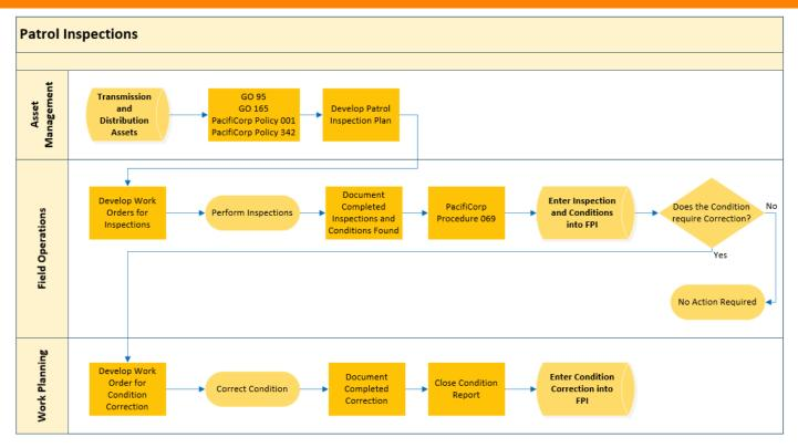
Figure 8-1 Patrol Inspections of Transmission and Distribution Electric Lines and Equipment
