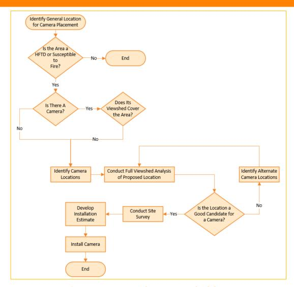
Figure 8-20 Camera Placement Methodology
