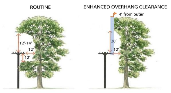
Figure 8-13 Enhanced Overhang Clearance
