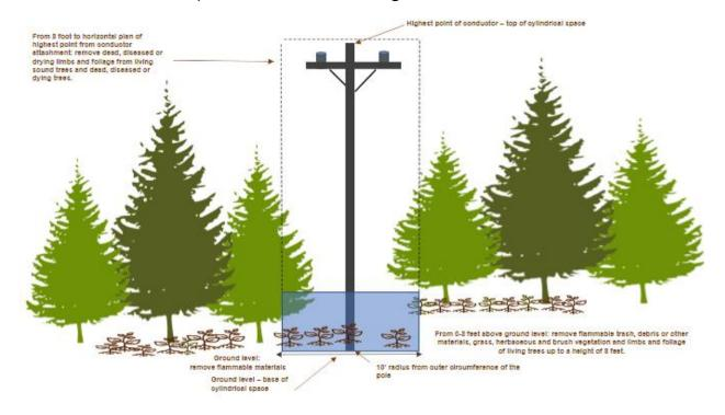
Figure 8-12 Pole Clearing
