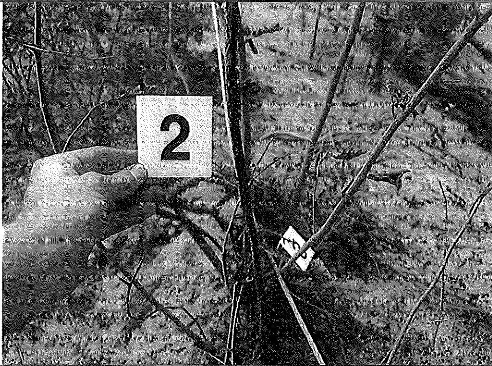
Photograph Number: 20 Electrical Date: 9/12/20 Time: 1355 Photographer: b6 & b7C Subject: Charred Conductor Struck Vegetation
