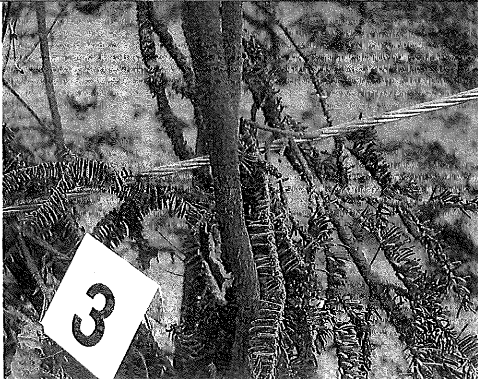
Photograph Number: 21 Electrical Date: 9/12/20 Time: 1356 Photographer: b6 & b7C Subject: Charred Conductor Struck Vegetation
